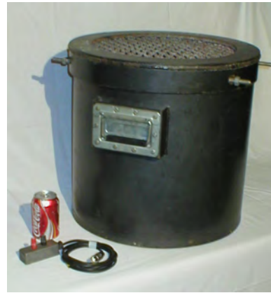
Bomb Tank & terminal lead
