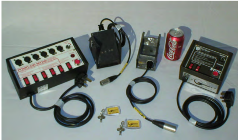
(left to right) 6-way Detonator, Angled Flash Box, Standard Flashbox and 2-way Detonator
